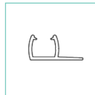
6mm Vertical Flap with 15mm Leg PGFVL15-6
